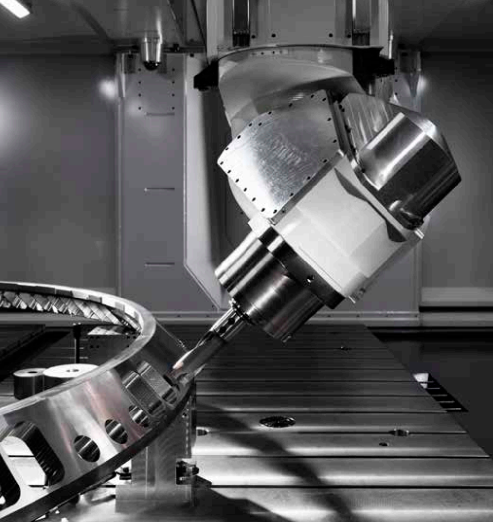
Machining of slewing bearing
