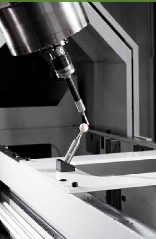
5-axis calibrating station
